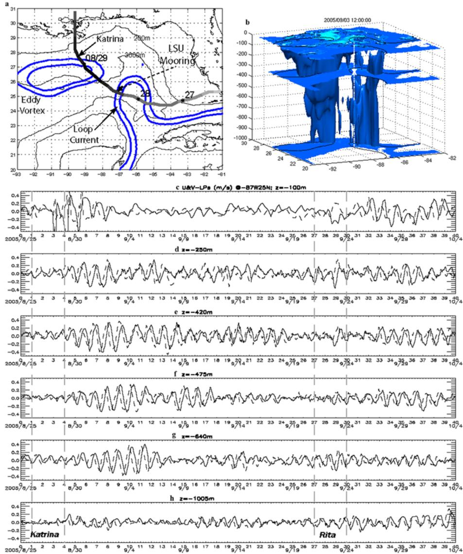
**Figure 1.** (a) Study area showing mooring location, Katrina track (dark indicates wind speed  $>60$  m/s), and the thick contours are SSH = 0, 0.2 m. (b) The 3-d surface of inertial energy =  $0.03 \text{ m}^2 \text{ s}^{-2}$  on Sep/03/12:00. (c)–(h) Observed high-passed  $u$  (west-east; solid) and  $v$  (dashed) velocities (m/s) at the mooring at the indicated depths, during hurricanes Katrina (Aug/26~29) and Rita (Sep/21~24).
