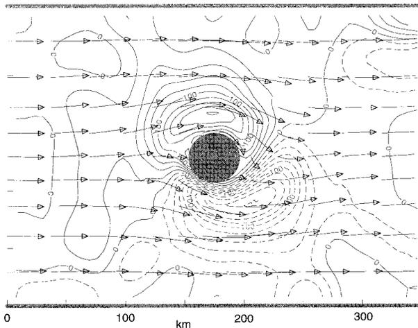
FIG. 6. The full nonlinear model with a throughflow of  $0.20 \text{ m s}^{-1}$  applied uniformly at  $x = 0$ . The diffusivity is nil. Shown are the differences between the densities at day 2 and the initial densities at a depth of 2000 m. Contour interval =  $20 \times 10^{-4} \text{ kg m}^{-3}$ . The arrows represent particle trajectories for 2-day flights based on instantaneous Eulerian velocities. The model ran successfully for 30 days with no sign of numerical instability.
