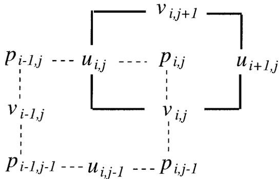
FIG. 4. The stencil for a C grid. (a) The solid box denotes the principal grid cell. (b) The dashed box denotes the offset cell used to finite difference vorticity. The variables  $H$  and  $b$  are collocated with  $p$ .
