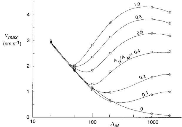
FIG. 7. The maximum velocity error as a function of the horizontal viscosity  $A_M$  ( $\text{m}^2 \text{ s}^{-1}$ ) and the ratio  $A_H/A_M$ . Here  $S = 4$  and  $t = 10$  days. Computations were made at the circled points.
