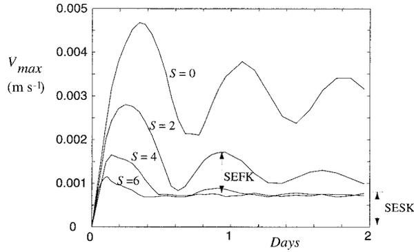
FIG. 3. The maximum velocity as a function of time for the case  $r_{\max} = 0.211$ . These are fully prognostic results. If run diagnostically ( $b'$  held constant), then  $V_{\max}$  would be identical to the case for  $S = 0$ ; this would also be true for other values of  $r_{\max}$ . The singular behavior of the  $S = 0$  case is explained in appendix A.
